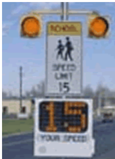
4 – School Radar Sign
